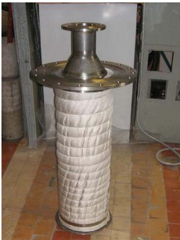
Fig. 6. External view of the GFC radial bed for incineration of chlorinated hydrocarbons.
